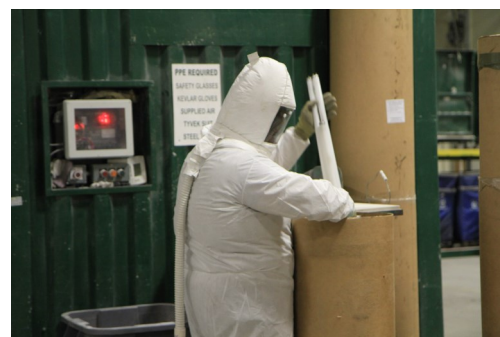
"Michelin Man" ventilated suits protect workers loading lamps into crusher from mercury on phosphor powder and glass dust.
